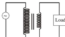
The e.m.f. of secondary coil is less than that of primary  $E_s < E_p$ .
