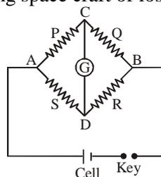
two junctions as shown in the diagram. If three of the resistance P,Q,R are known, the fourth (S) can be determined. Keeping the resistance P, Q fixed the resistance R is varied till the galvanometer shows zero deflection. When this is achieved  $\frac{P}{Q} = \frac{R}{S}$ . For maximum sensitivity all the four resistances should be of the same order.
